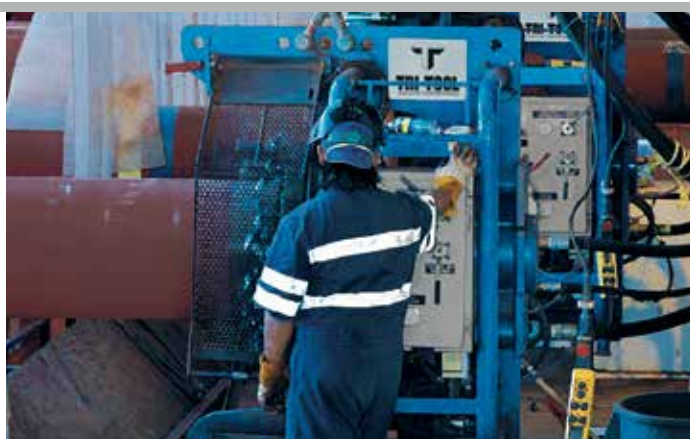
The operator of the PFM 1632 is using the on-machine controls versus the full function pendant control (shown).
