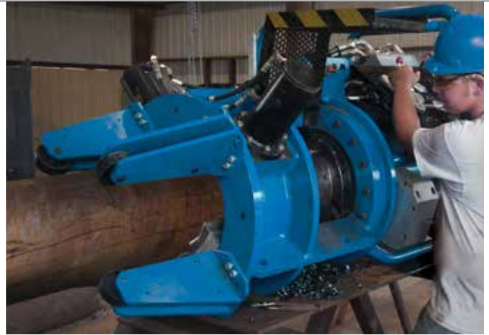
A PFM 614 utilizes a set of adjustable stationary locator pads that are opposed by a set of powerful clamping pistons that provide rapid, secure clamping.
