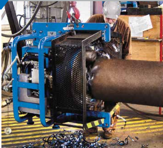
The high speed PFM 816 demonstrates the machine's optimal cutting ability (and the safety chip guard) by the long blue chips produced by the cut.
