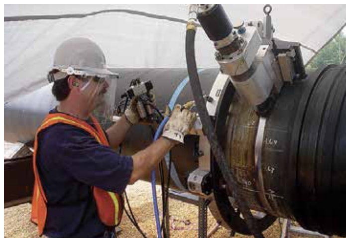
This WPS shows the ability to mount in-line on a welded pipe and produce a smooth transition across the weld prior to re-coating for corrosion control.
