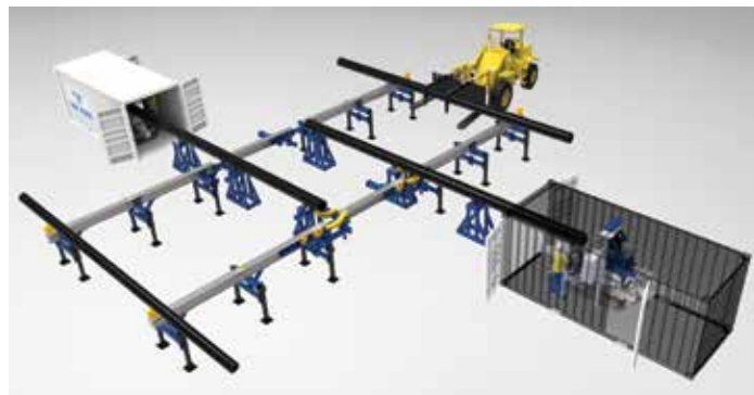
Tri Tool's Counterboring Service is performed on a fully mechanized pipe rack, designed to ensure for maximum safety and high-performance cycle times
