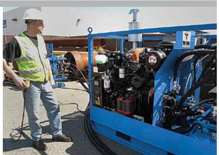
A diesel powered HPU providing hydraulic power to a PIPEMASTER PFM 1632. The HPU unit is fully controlled by means of the operator pendant.
