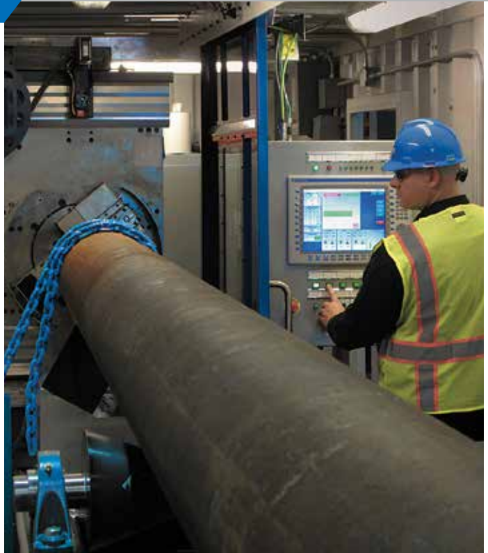
Two fully automated work stations, one for each end of the pipe, provide true 7 axis machining for unprecedented control over the deep counterboring process.
