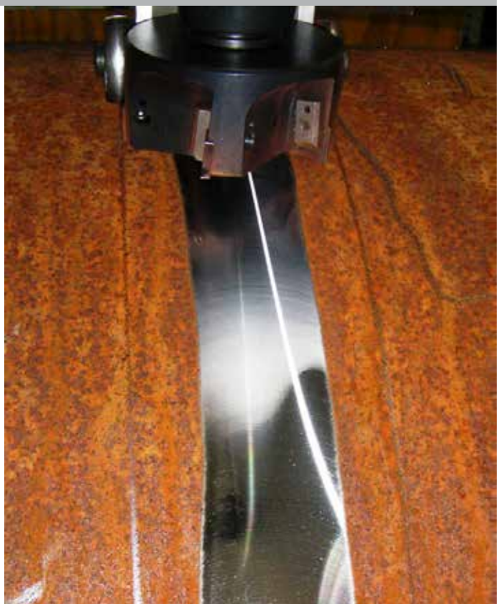
The almost mirror-like surface of the Weld Profiling System is a result of the stable Clamshell platform. Tracking wheels shown guarantee height control.
