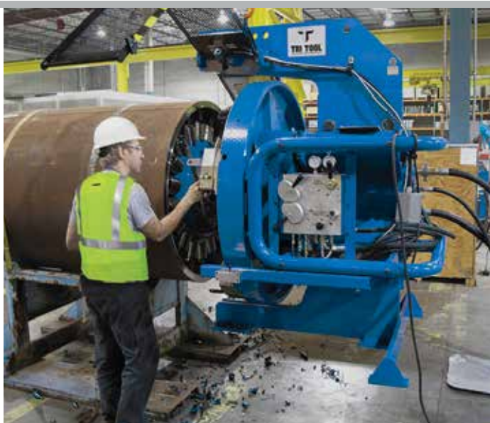
The solid construction of the PFM 3248 is key to its ability to produce perfect surface finishes despite the high rotation speed of the massive cutting head.
