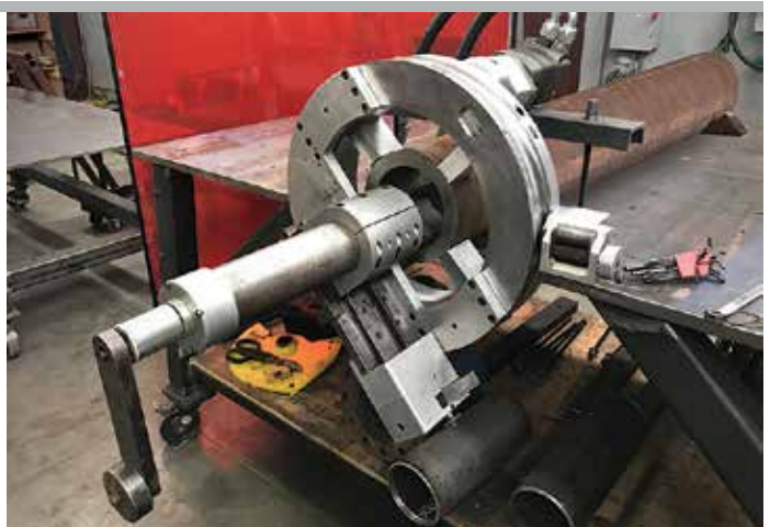
Tri Tool's 600 Series SB and TRIMAX Clamshell lathes provide a stable and secure platform for precision counterboring, an absolute necessity for effective pipe matching and testing.
