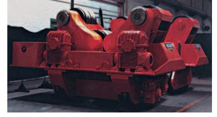
Bode's Traversing Self-Aligning Rotators follow the well established reputation of their static counter-parts for ease of use and reliability.
